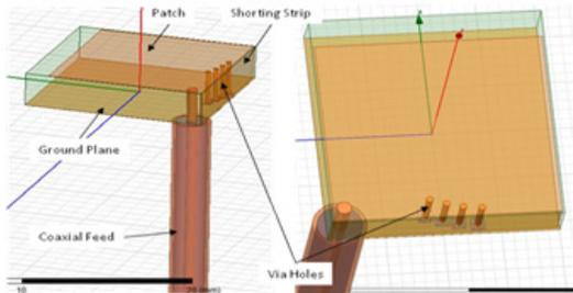
Figure 2: A half-patch antenna with one shorted edge containing four plated through via holes between the top patch and the ground.
