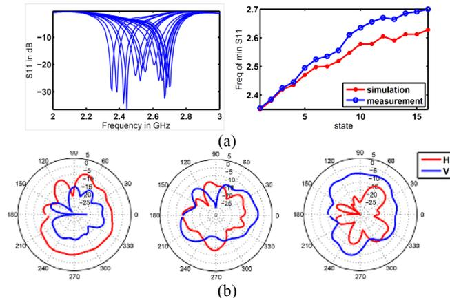
Figure 4: (a) Measured S11 and the measured frequency of minimum S11 for all sixteen logic states, and (b) measured gain patterns (dBi) for the 0111 state at 2.591GHz in all three cuts.
