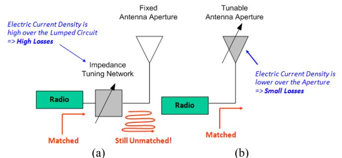
Figure 1: Difference between (a) Impedance Tuning and (b) Aperture Tuning.
