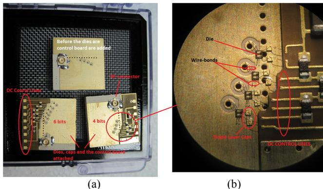
Figure 3: (a) 6-bit and 4-bit versions of the prototype built (view from the side of the ground plane) and (b) close up view of the bare-die switches wire-bonded to the antenna board and the DC control lines.
