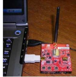
Fig. 8. ZigBee Setup with monopoles on both units.
